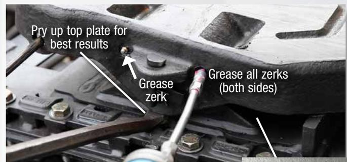
**Grease the mounting brackets.** Lift the top plate up with a pry bar to ensure grease gets to the top of the brackets. (Inspect mounting bracket base, and if "LUBE FREE" is cast into the bracket skip this step. These models have bracket liners and do not require lubrication. In this case inspect linings for wear). **In cold weather applications please refer to technical bulletin TB-008 and LT-203. Literature is available at [fifthwheel.com](http://fifthwheel.com).**
