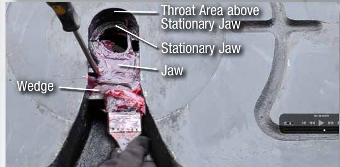
Separate the jaw and wedge with a screw driver and press the recommended lubricant between the serrated surfaces. Work the pull-handle back and forth to spread the lube over all surfaces. Also grease the Stationary Jaw and the Throat Area above the Stationary Jaw.
