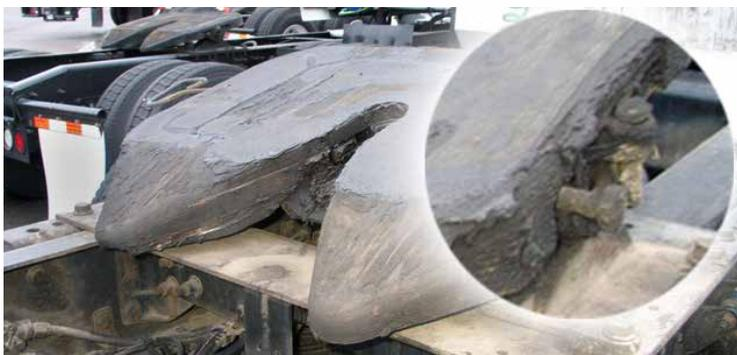
Over-lubrication is costly and causes excessive build-up on fifth wheel components leading to lost revenue.
