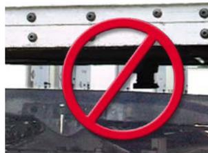
*Never inflate the suspension airbags when fifth wheel is below the trailer.*
