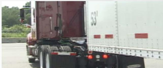
**EASE OUT FROM UNDER THE TRAILER.** Pull forward slowly until the fifth wheel clears the kingpin. Dump the air from the tractor suspension, and drive carefully away from under the trailer.
