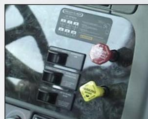
Open fifth wheel with release valve located on the dash or in a lock box mounted on the rear of the cab. To open, set the tractor parking brake and pull the release valve. Hold the valve open until the locking mechanism is locked in the
