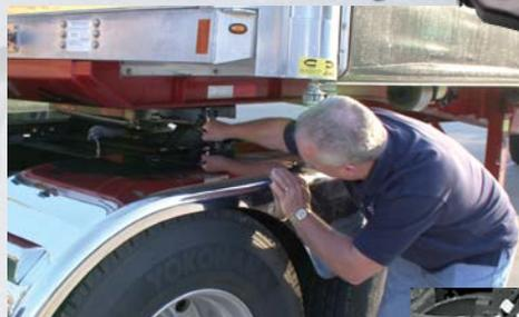
**DISENGAGE LOCK.** Release the fifth wheel lock by pulling the handle.
