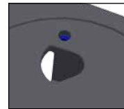
Air cylinder bolt access (under wear plate)
