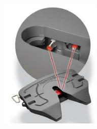
Figure 2: SmartLock fifth wheel
