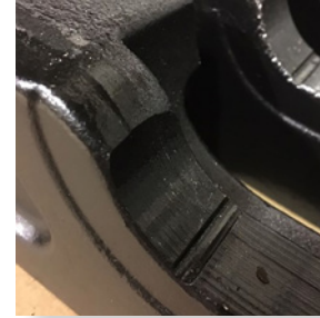
Wear grooves built into the Fontaine ARMOR locking jaw.
