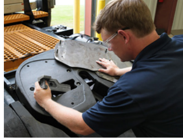
Technician removes a wear plate to rebuild the fifth wheel from the top side.
