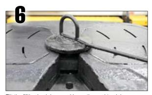
Tilt the fifth wheel down and lower the yard truck boom.
