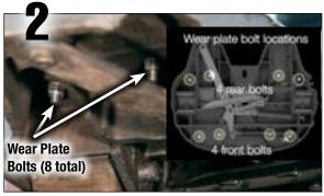
Install the eight wear plate nuts and washers. You can tilt fifth wheel up and down for easy access. Note all bolt locations in photo.
