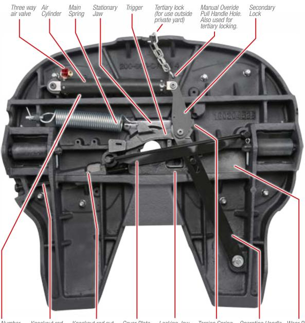
Serial Number Knockout rod Cover Plate Locking Jaw Torsion Spring Operating Handle Wear Plate Knockout rod nut (Behind air cylinder)
