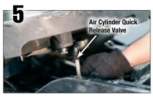
Connect the air hose to the air cylinder quick release valve.
