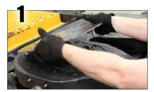
Install both wear plates. Apply grease to top surface.
