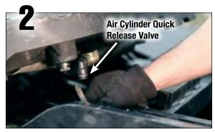
Raise the yard truck boom for easy access, then remove the air hose from the air cylinder quick release valve.
