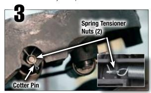
Remove two spring tension by removing the cotter pin with pliers. Then remove the two spring tensioner nuts. **Hint:** You can place a screwdriver in the main spring loop to prevent spring from rotating when unbolting nuts (see video).
