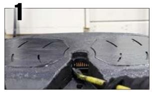
Trip the wheel closed using a crowbar. **NEVER use hands to trip an activated fifth wheel.**
