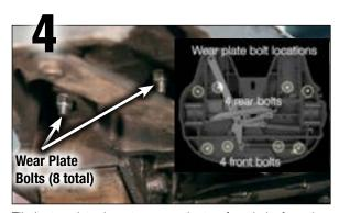
Tilt the top plate down to access the two front bolts from the opposite side of the top plate. Remove the eight wear plate nuts and washers. Note all eight nut locations in photo.
